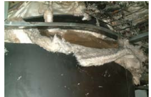
Muffler – the elevated deformation due to muffler explosion is evident
