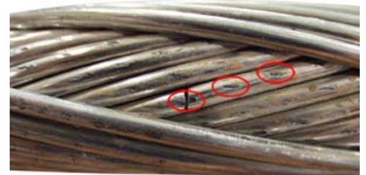
Visual analysis of the cable – the oval spots made by fretting are evident.
